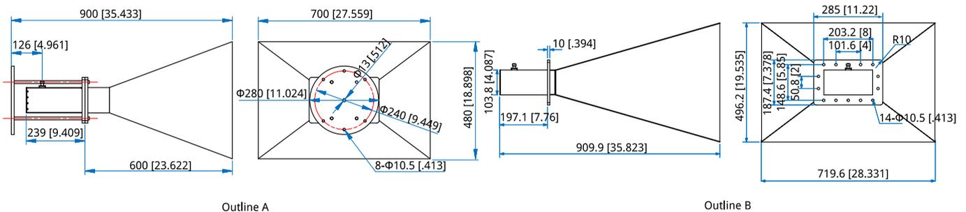
Unit: mm [in] Tolerance:  $\pm 0.2\text{mm}$  [ $\pm 0.008\text{in}$ ]
